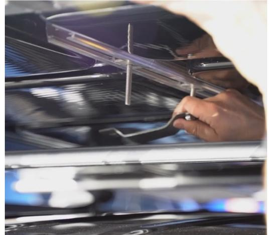
Step 7: Place each of the four mounting plates onto the two bolts at each corner and thread the included nuts onto the bolts (see photo next page - proceed to next step before tightening all the way).
