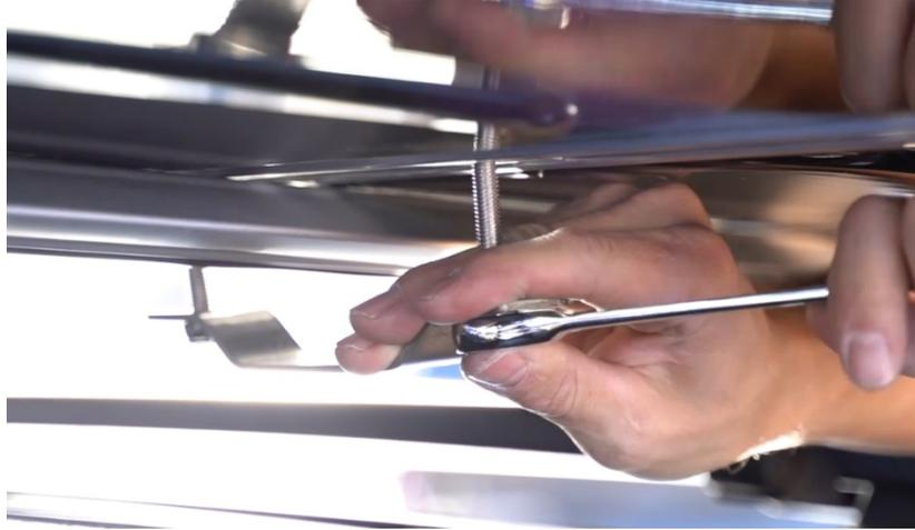
Step 8: Now it's time to orient the Roofnest so that it is centered where you want it. If the mounting hardware is loose then you should be able to move the Roofnest so that it is lined up on your roof where you want it.
