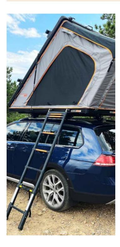
Roofnests are engineered to be mounted to two crossbars that are at least 30 inches apart. Platform racks can be used, but are not necessary and in some cases make installation trickier.
